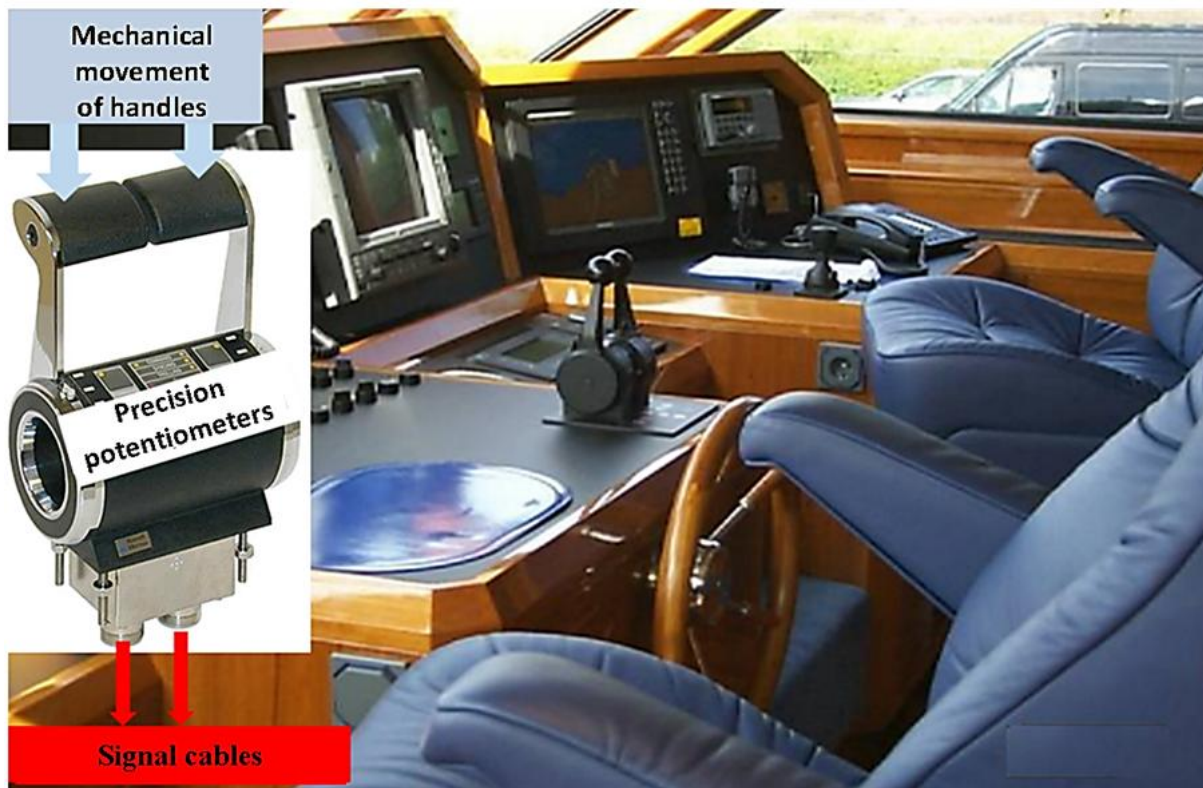
Figure 8. The navigator's console and the command unit of the Mini-Marex remote automatic control system
