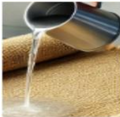
Figure 7. Mat Water Permeability Test
