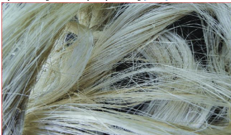
Figure 3. Extracted Enset Fiber (Image Camera resolution, 100MP)
