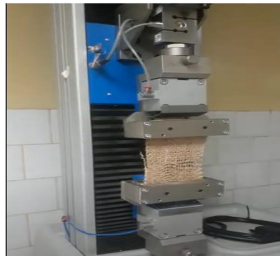
Figure 5. Tensile Strength testing of Enset Fiber Mats
