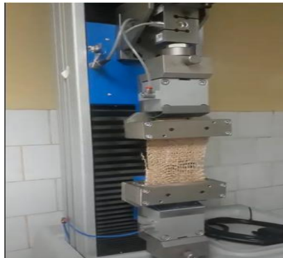
Figure 5. Tensile strength testing of enset fiber mats.
